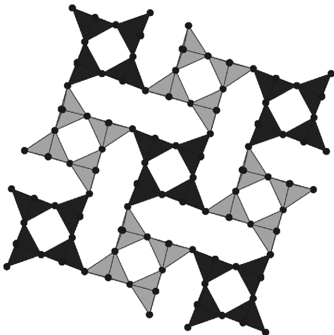
FIG. 7. Magnetic structure of \text{Sr}_2\text{MnO}_{3.5} . Spin-up polyhedra in gray; spin-down polyhedra in black.
